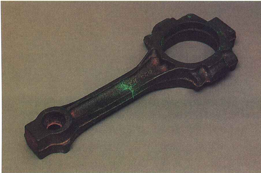
Figure 5. Water-based medium is used for connecting rod inspection. Defects like the one seen here stand out with no confusing background.
